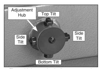
Figure 64. Lower wheel adjustment control.
